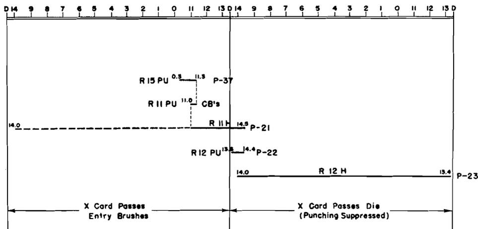
Figure 49. Sequence of Operations on Punch Suppression
