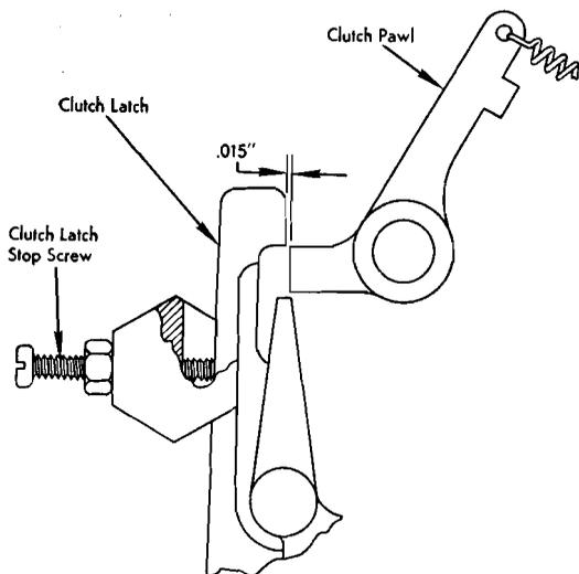
Figure 29. Clutch Adjustment
