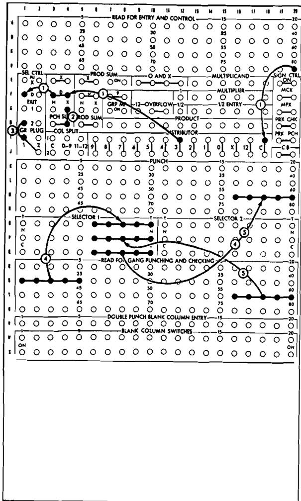
Figure 5. Use of Class Selector for Offset Gang Punching
