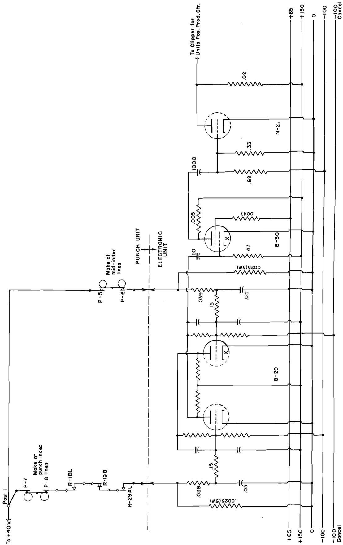
Figure 127. Product Counter Read-out Pulses
