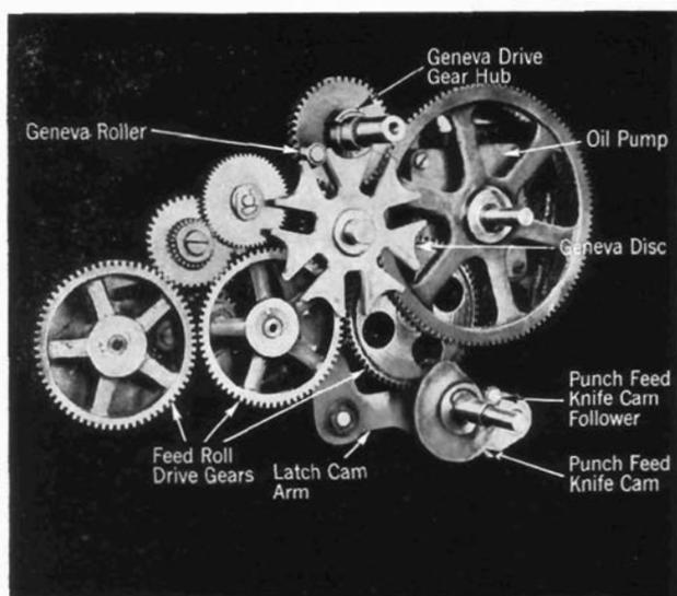
Figure 19. Geneva Mechanism
