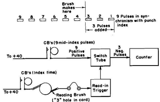
Figure 95. Block Diagram of Counter Read-in Circuits
