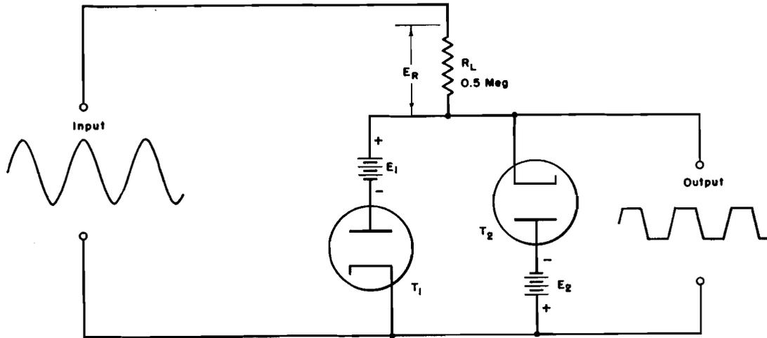
(A) Diode Peak Clipping Circuit
