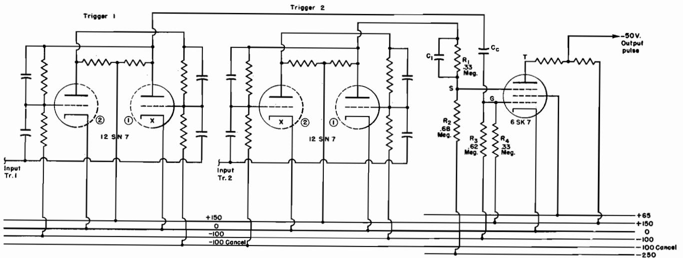
Figure 88. Control of Pentode Switch with Two Triggers
