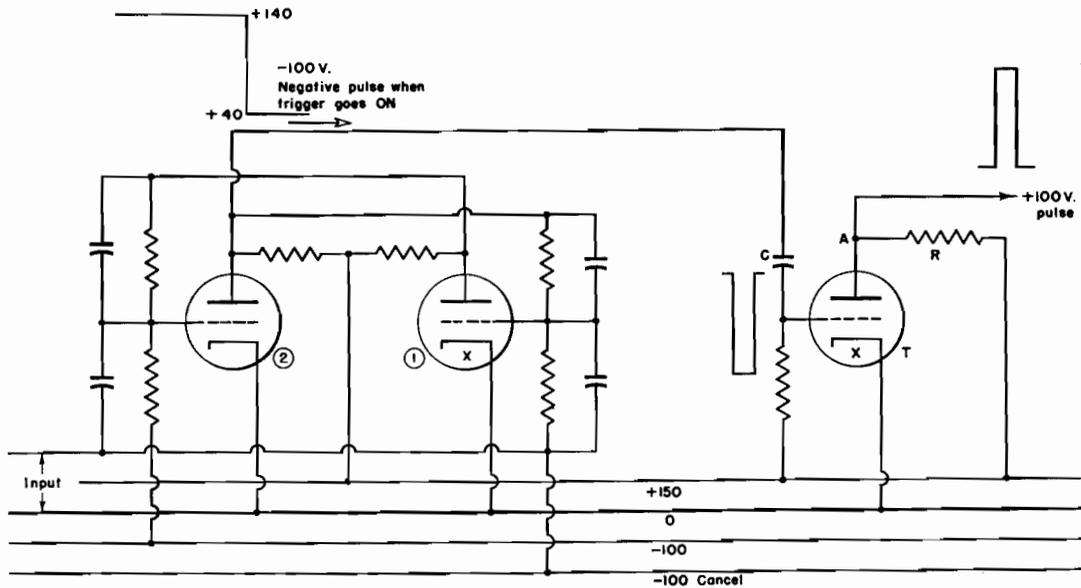
Figure 86. Use of Trigger to Control Triode
