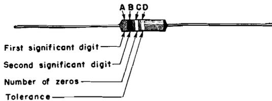
(A) Resistor Color Coding (Values in ohms)
