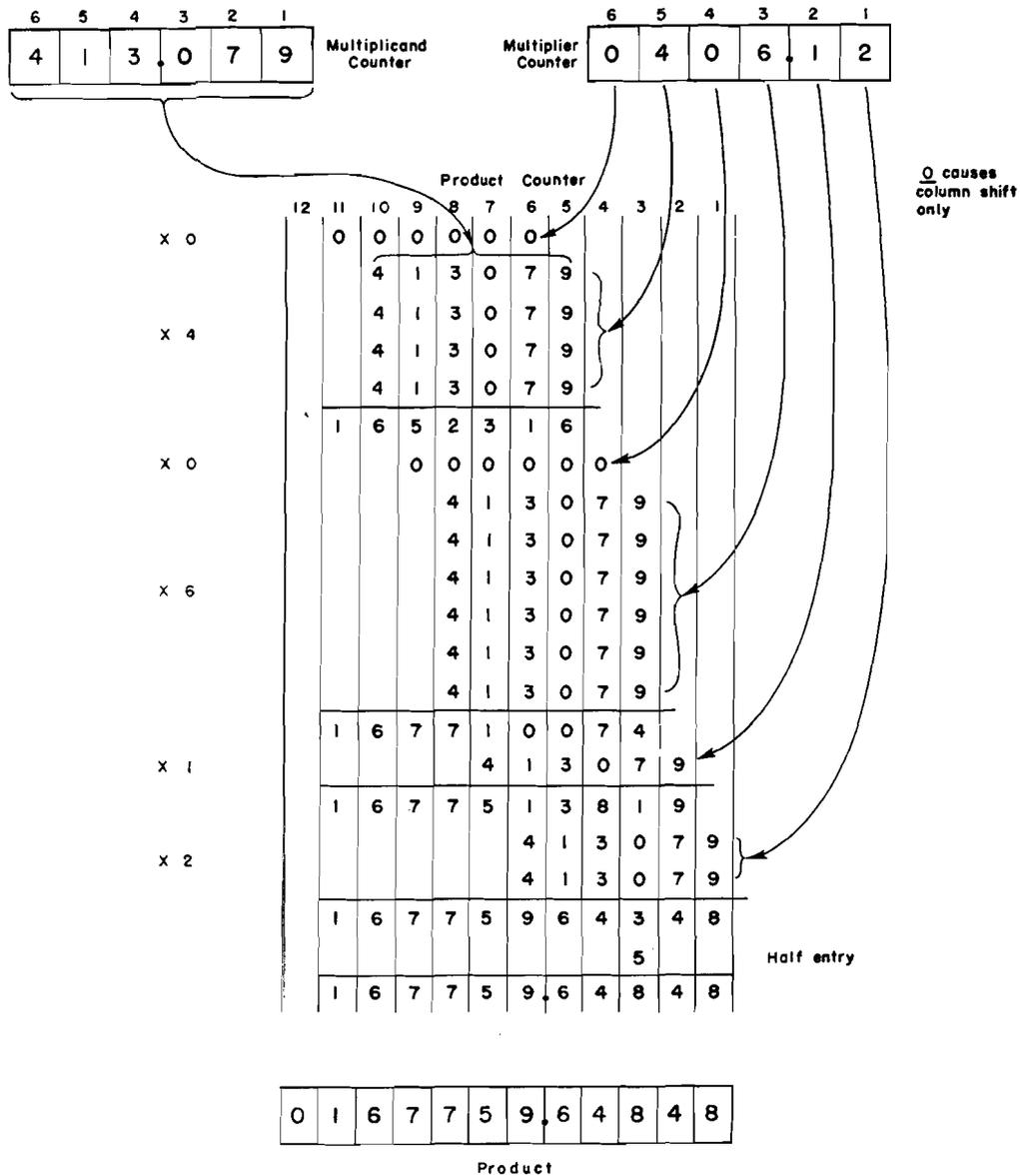
Figure 58. Principle of Multiplication
