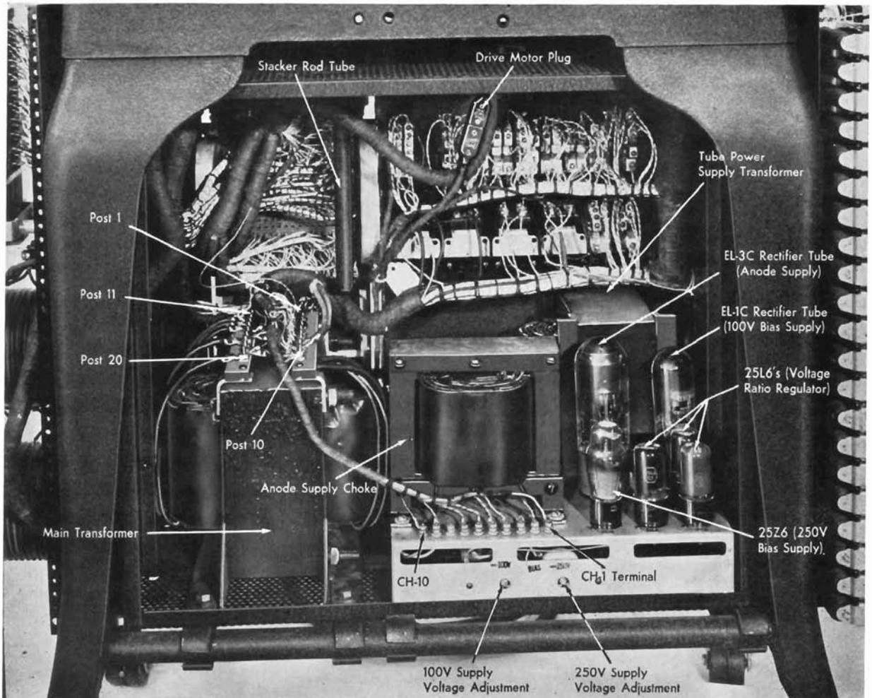
Figure 11. Closeup of Main Transformer and Tube Power Supply Chassis
