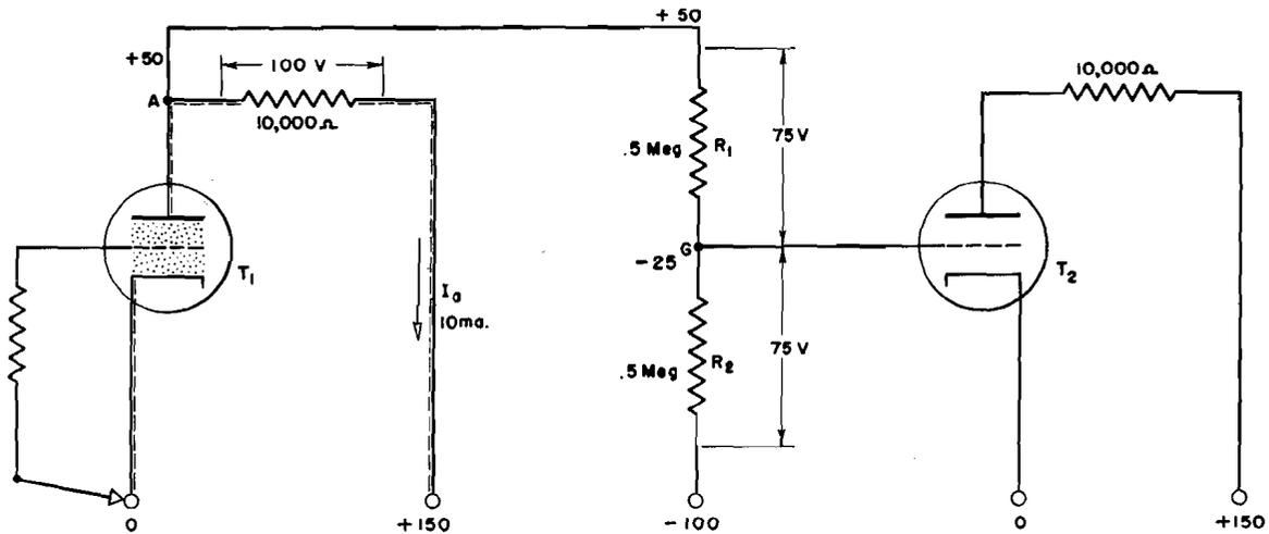
Figure 69. Direct-Coupled Triodes
