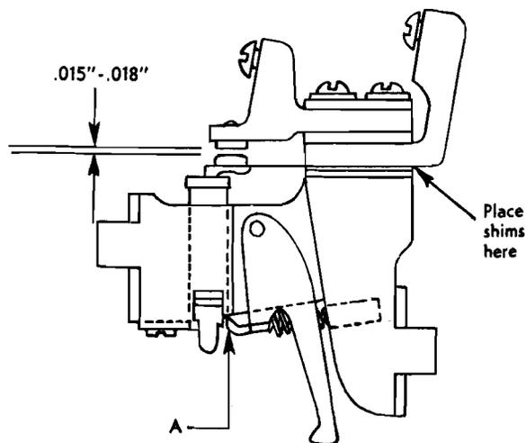
Figure 43. Circuit Breaker Adjustment
