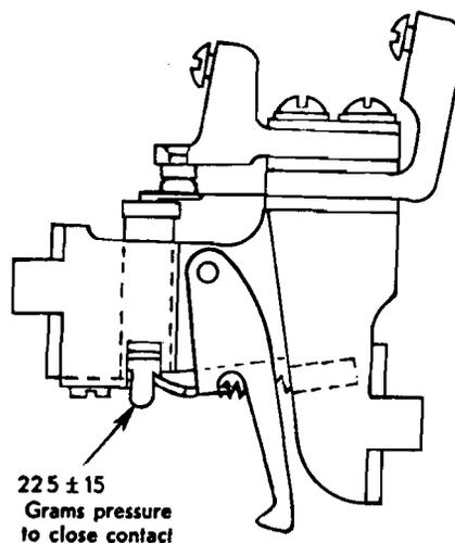
Figure 44. Circuit Breaker Adjustment
