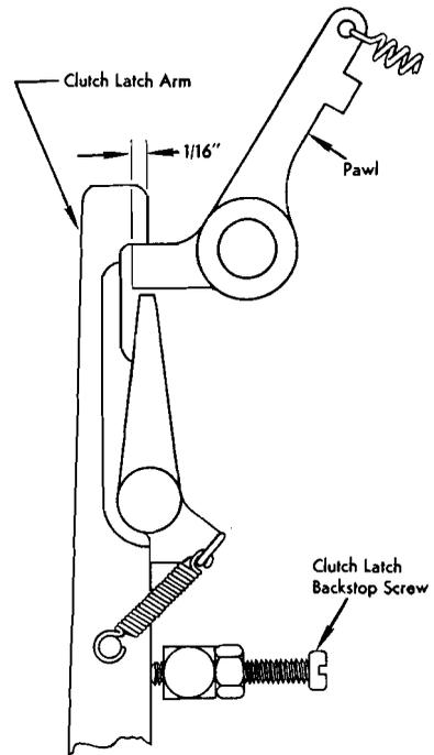
Figure 30. Clutch Adjustment
