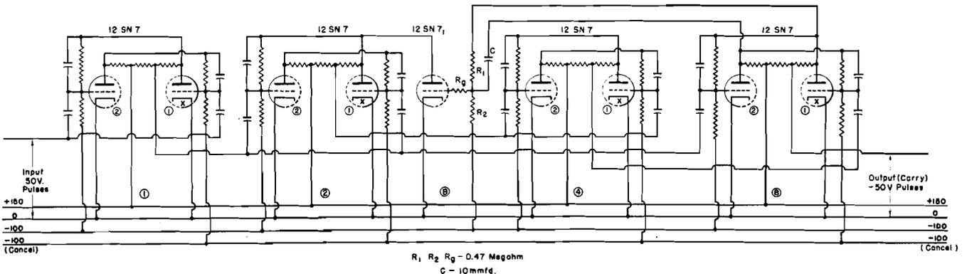
Figure 90. One Position of an Electronic Counter
