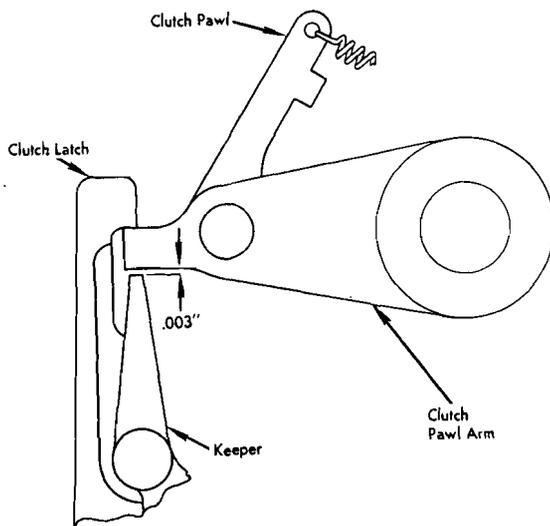
Figure 32. Clutch Adjustment
